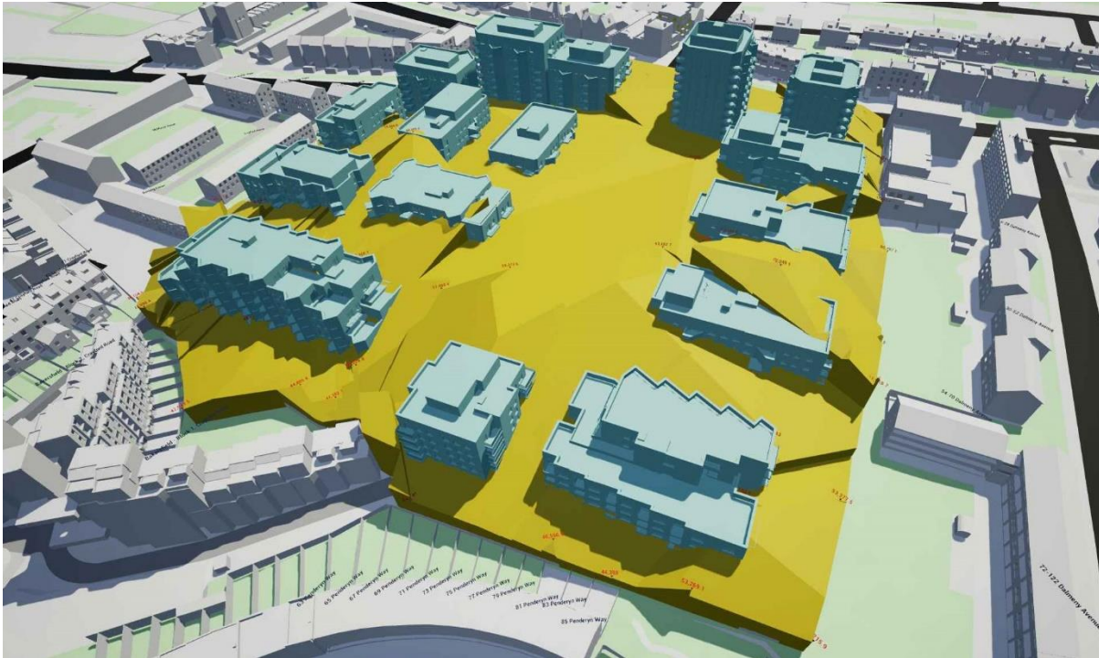
Figure showing the extent of a BRE compliant massing to the site
