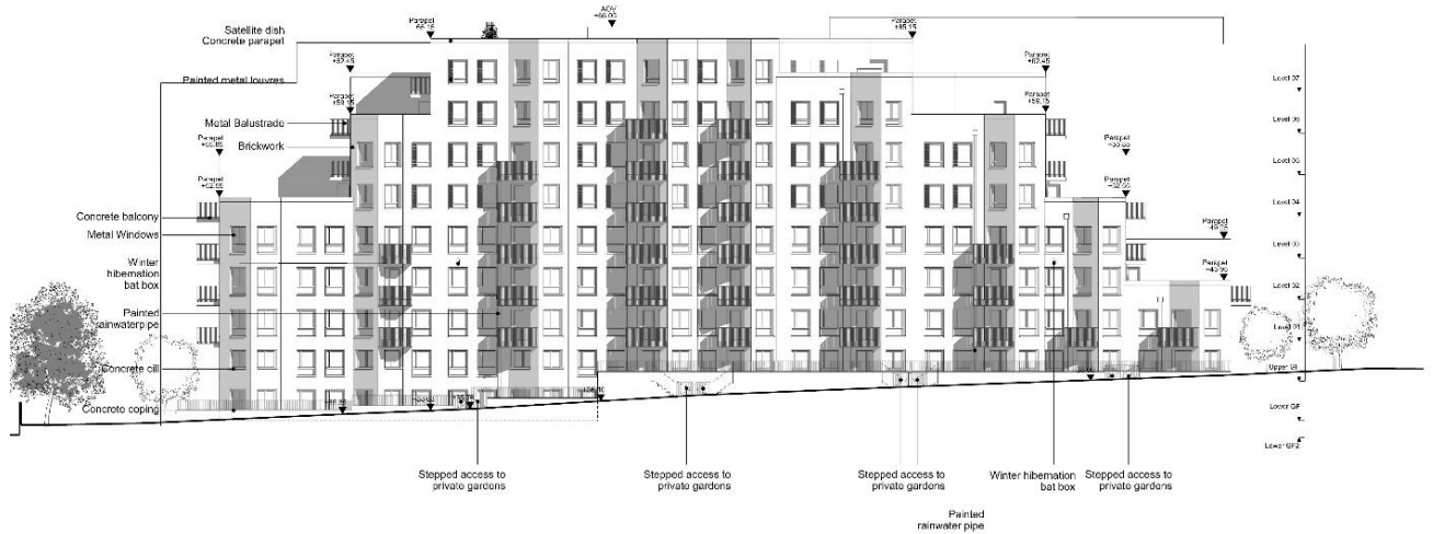
Figure 1.20: A1 / A2 - North west elevation
